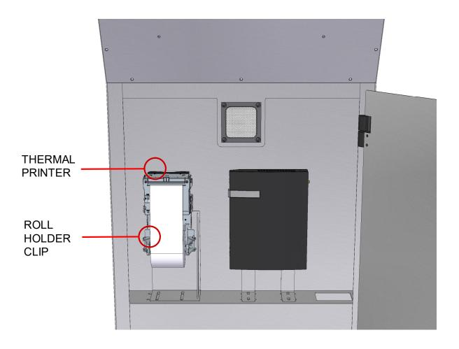
In the versions of the kiosk supplied with integrated panel devices (thermal printers, card readers, banknote acceptors) it is possible to easily inspect these devices by opening the rear door.
